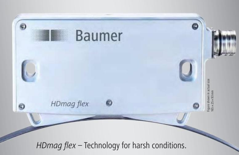
HDmag flex magnetic belt encoders operate on the proven HDmag principle which is based on high-resolution magnetic sensing by precision material measure with real time signal processing. The sensing head provides two adjustable sensing elements which are aligned in the factory to match any required shaft diameter. The ultra-precisely encoded magnetic belt is simply buckled on the shaft.
